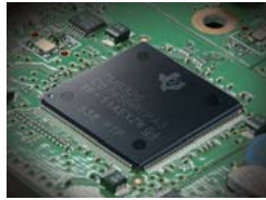
32-bit floating point IF DSP
